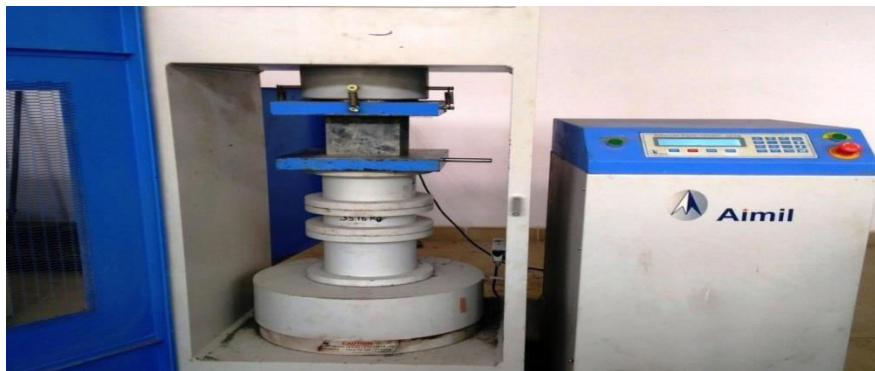
Fig .2.4 The Compressive Strength Test on Machine
