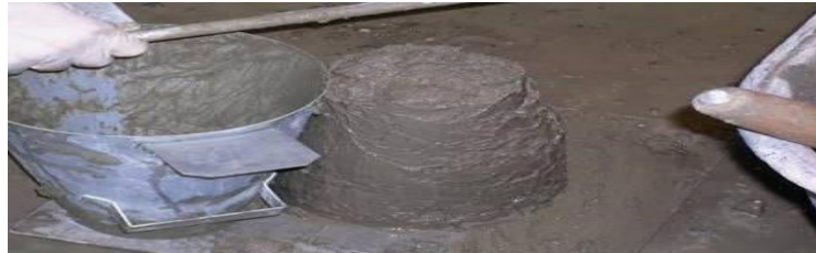
Fig.2.3 Test of Concrete slump
