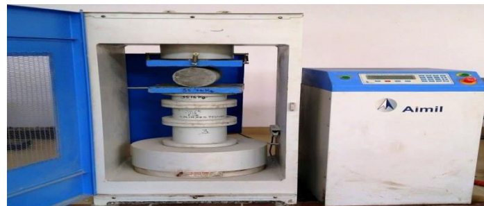
Fig.2.6 Concrete Splitting Tensile Strength Test
