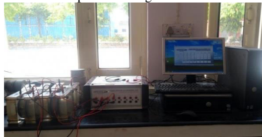
Fig .2.9 Chloride-ion Permeability test
